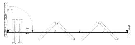
**Side Stack** There is a main, straight line of track, with the stacking area mainly off to one side of the track only (looks like an h shape). The panels run along the main line of track and turn perpendicular to the track. The carriers/trolleys move 95% to the side of the centreline of the head
