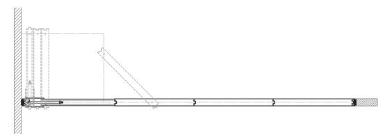
**Remote Stack** There is a main, straight line of track, with the stacking area completely off to one side of the track only (looks like a one-handed Trident/pitchfork). The panels run along the main line of track and turn perpendicular to the
