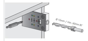
The Grass drilling jig for Soft-close can be used for drilling all adapter plate versions and the drill-in damper
