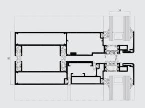
CW 86 enables cassette façades to be built using a traditional stick structure (CW 86). It also enables unitised façades (CW 86-EF) to be completely pre-assembled in the workshop that results in a high execution speed on the building site.
